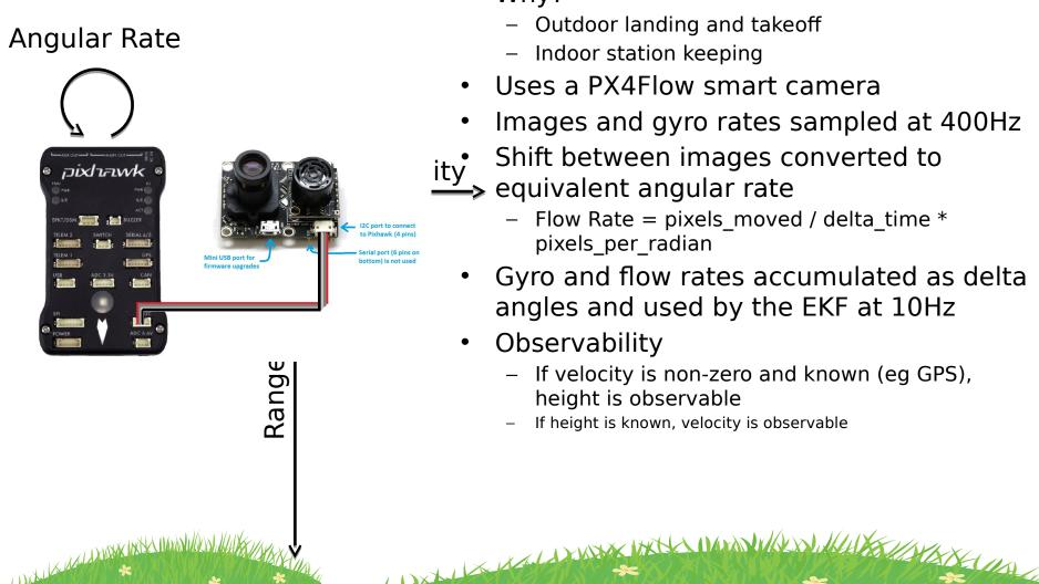
Flow rate = Angular Rate + Velocity / Range
