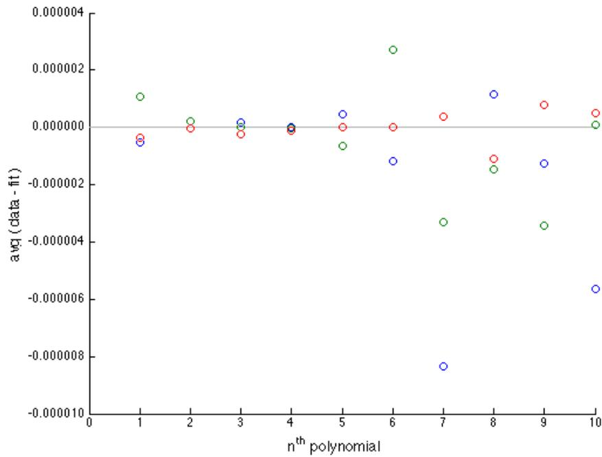
Deviation of average error of polynomial fit (gyroscope: radians / second):
